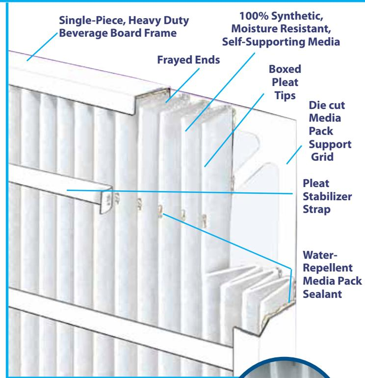
*Consistent pleat shape and spacing allow particulate to collect evenly over the entire surface of the media. Pleat stabilizer straps add rigidity and maintain proper pleat spacing. Opposite photo of air leaving side shows the integral media pack support grid.*
