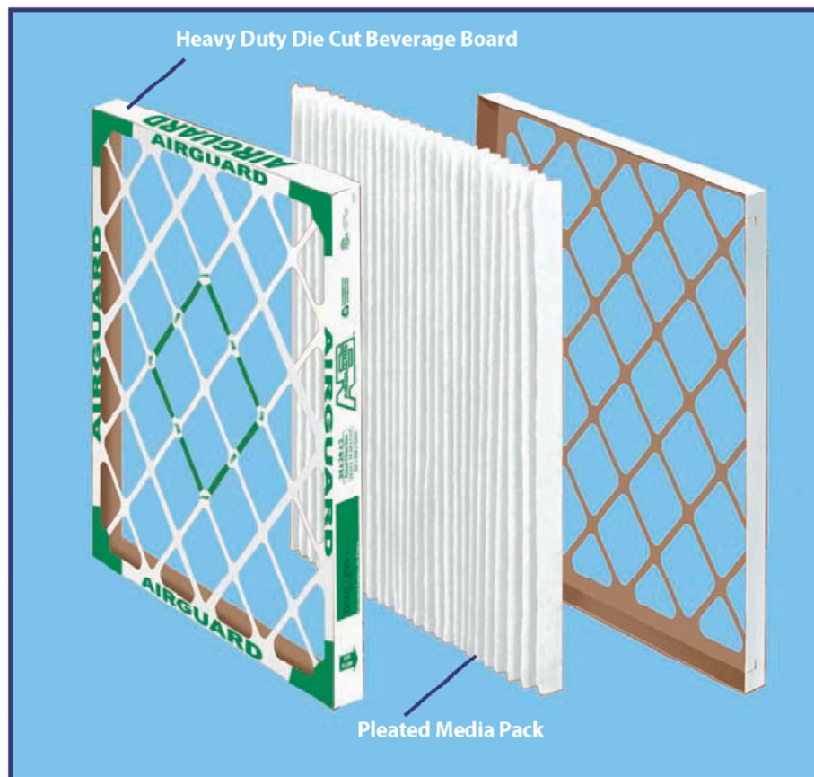
Two mating pieces of die cut beverage board form a double wall frame around the perimeter of the filter. DP filters will not rack or warp under normal operating conditions.
